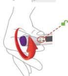
**Unlock** by turning the lock ring toward the unlock icon.
